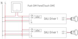
Remark: Only use open push button without indicator light. Maximum cable length between each Unit: 20 meters.
