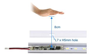
Hold your hand in front of the sensing head for more than 2 seconds: The brightness increases or decreases continuously, the each time the hand is removed and then held again, the brightness changes in the opposite direction.
